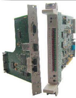
The OMI (OMNEO Matrix Interface) card set for RTS ADAM and ADAM-M intercom frame provides fully IP compliant connectivity into the ADAM intercom BUS for OMNEO compatible devices. The card set consists of a back card and front card and supports fiber optic cabling (through the use of optional fiber modules) and RJ45 copper Ethernet connections.
