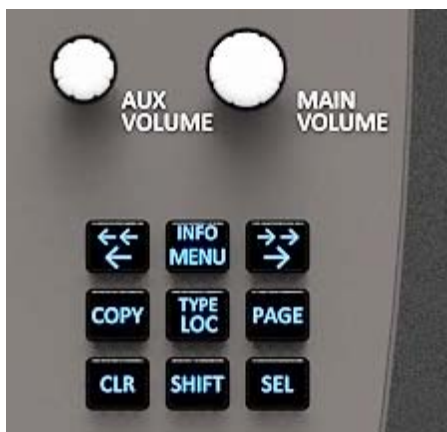
FIGURE 6. DKP-3016 shaft encoders
