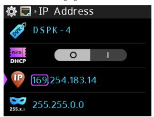
3. Rotate the **B/D shaft encoder** to make changes.
