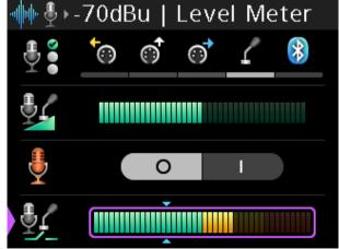
**NOTE**: The blue arrows indicate the current noise level. You want to set the noise gate just above the current noise level.
