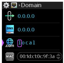
3. Rotate the **B/D shaft encoder** to scroll through available characters.
