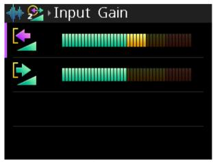
3. Rotate either **shaft encoder** to adjust the level.
