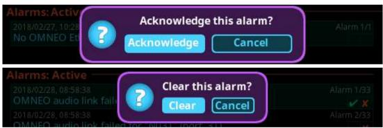
When viewing all alarms and pressing SHIFT+SEL buttons (or SHIFT+Right-click) prompts to Acknowledge All or Clear All (clearable) alarms at once.
