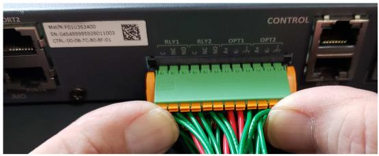
Figure 7.1: 24-position Terminal Block Connector
