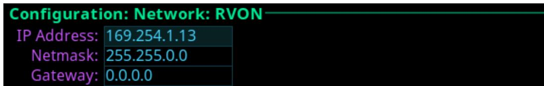
Figure 21.4: Configuration | Network | RVON
