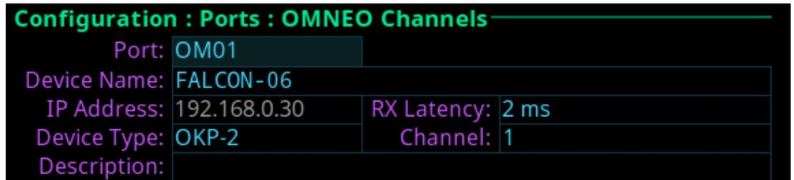
Figure 22.6: Configuration | Ports | OMNEO Channels
