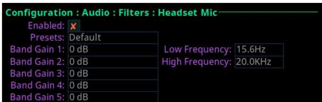
**Figure 23.6:** Configuration | Audio Filters | Headset Mic
