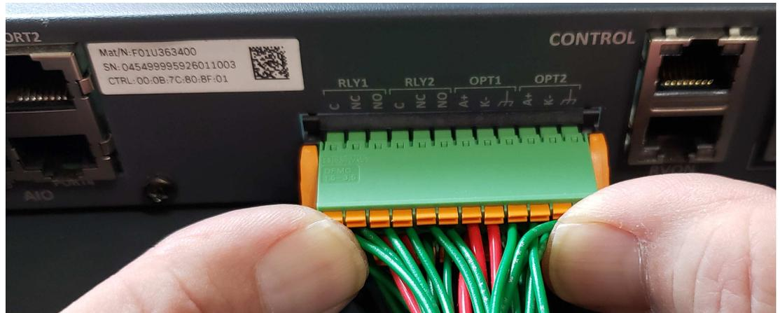
**Figure 7.1:** 24-position Terminal Block Connector
