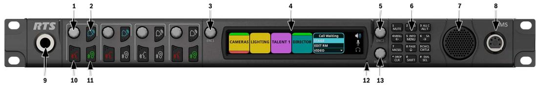
Figure 4.1: OMS front panel reference view
