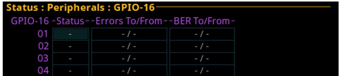
Figure 16.2: Status | Peripherals | GPIO16 Screen
