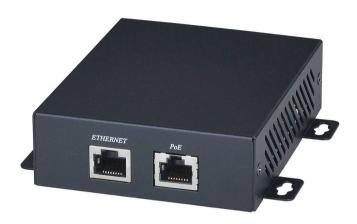
The PoE Power Kit for the AP-1800 is a full 60W, industrial, PoE (Power over Ethernet) splitter solution that splits out DC power from the DC + data of the Ethernet network, which eliminates the need for a local power supply. This add PoE functionality to non-PoE devices that have a power consumption up to a full 60W. The PoE splitter is perfect for network devices that need higher power.
