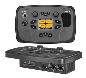
The **DSPK4** (Digital Speaker Station) is an IP-based version of its wired analog speaker station predecessor, with several key enhancements, such as high quality digital audio and the use of standard Ethernet, making it compatible and versatile to fit into any environment.
