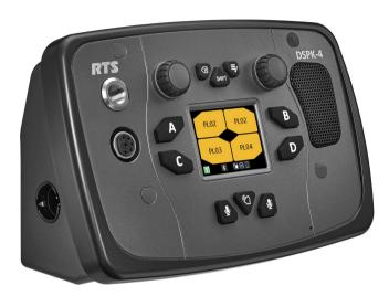
The **DSPK4** (Digital Speaker Station) is an IP-based version of its wired analog speaker station predecessor, with several key enhancements, such as high quality digital audio and the use of standard Ethernet, making it compatible and versatile to fit into any environment.
