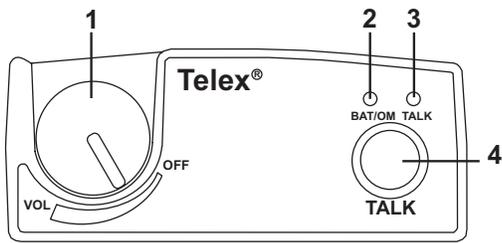
1. **On/Off & Volume Control** - Turns the beltpack power on and controls headset volume.
