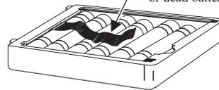
3. Load new batteries following the polarity as shown in battery case
