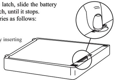
2. Pull battery strap to remove low or dead batteries.
