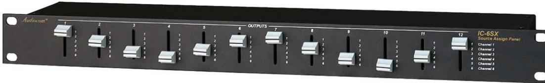
The IC-6SX is a 6 IN by 12 OUT routing switch. Six (6) channels of intercom from a master station can be assigned to any of 12 output lines. Output lines can go to almost any type or group of intercom stations, from single channel beltpacks to multi-channel user stations. Users can slide switches on the IC-6SX to different positions and combine or isolate any intercom stations in any combination.
