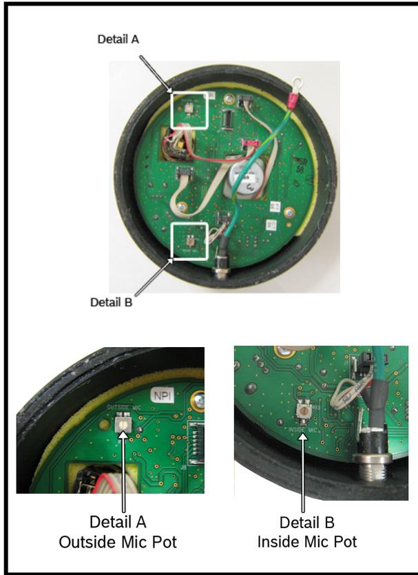
To **adjust the inside or outside mic sensitivity level**, do the following:
