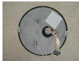
**CAUTION:** Do not allow the intercom to hang from the ground wire. The wire connection may break.
