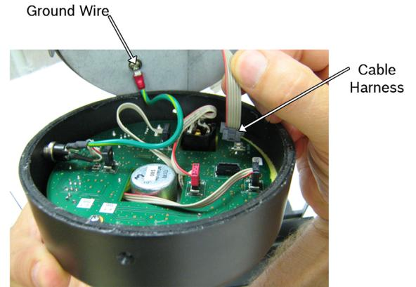
8. Attach the **cable harness** from the customer unit to the connector on the operator unit.
