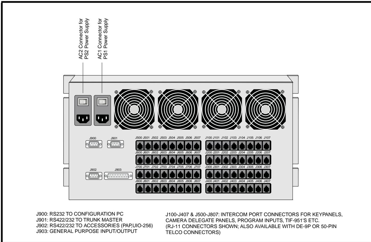
**FIGURE 16. ADAM CS Back View (Shown with RJ-11 Connector Panel)**
