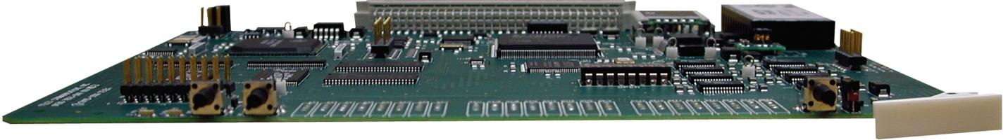
The RVON-C **VoIP** (Voice over Internet Protocol) card introduces all the VoIP functionality of the RVON-8 for ADAM, to the Cronus intercom system. The RVON-C converts analog audio to digital VoIP audio. Installed directly into Cronus, the RVON-C expands the connectivity to the Cronus intercom system by supporting eight (8) channels in and out. You can have up to four (4) RVON-C cards in Cronus at one time totaling 32 channels of VoIP audio plus data.
