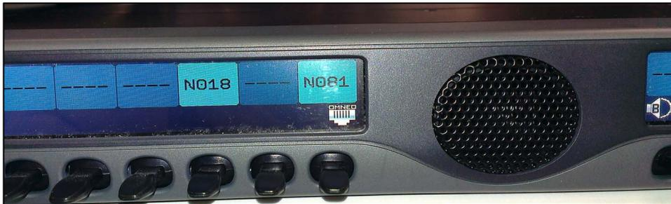
OMNEO enabled keypanel (*OMNEO Offers\Keypanel\AIO* set to *disabled*)
