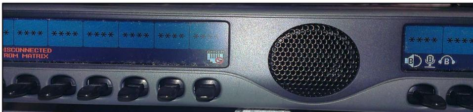
OMNEO disabled keypanel (*OMNEO Offers\Keypanel\AIO* set to *enabled*)
